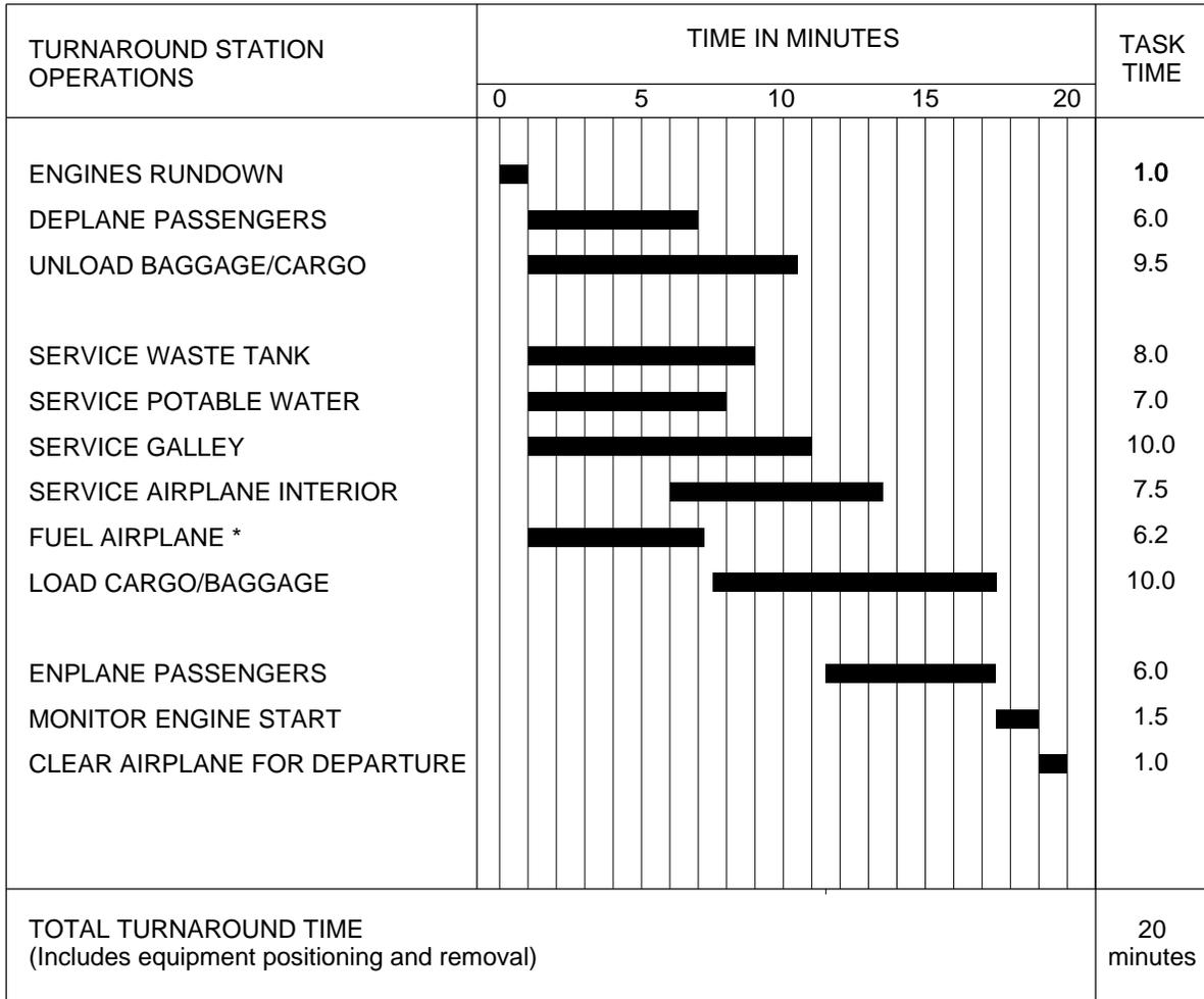
\* 85% FUEL UPLIFT, REFUELING PRESSURE 50 ± 5 PSI (344 kPa) AT 295 gpm (1136 Lpm).
